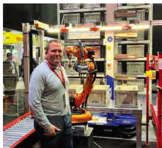
Christopher VanDeWiele, a product manager for MHS, pointed out how HAI's ACR robots bring goods to a Mujin robotic piece picking system, as part of MHS's new goods-to-robot solution.
