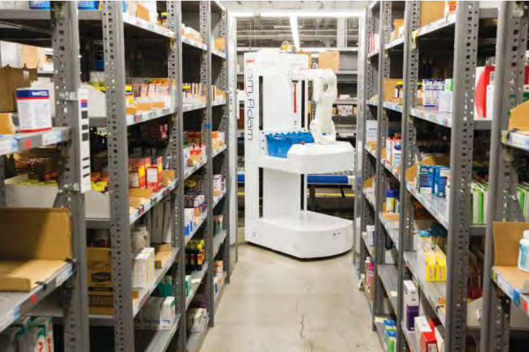
The mobile robot travels through the aisles in its zone and picks items for a store order to a tote.
