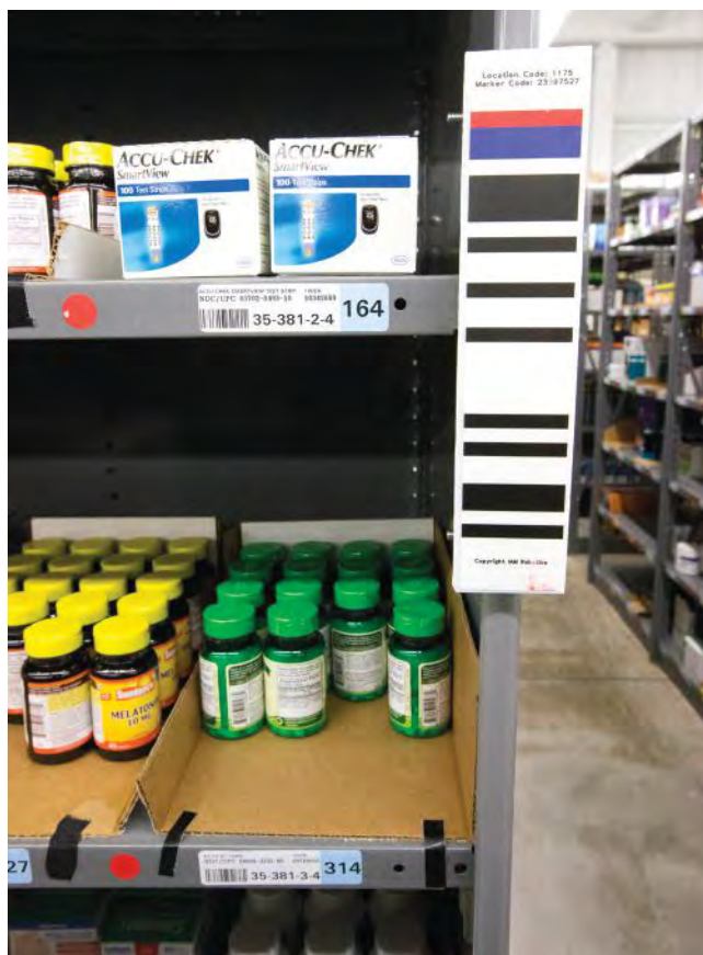
The robot reads end of aisle bar codes to navigate through the pick zone.
