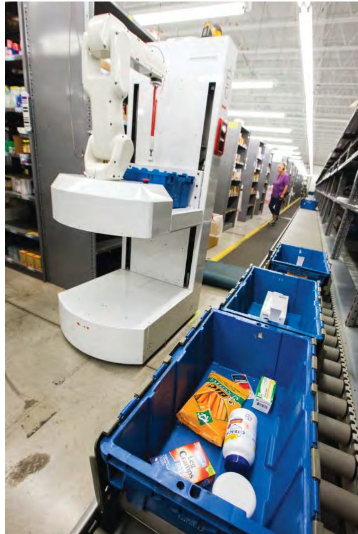
Once an order is completed, the robot travels to an induction station. For now, an associate inducts the tote onto the takeaway conveyor.
