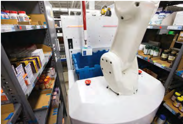
Once the robot reaches a pick location, it identifies the item to be picked. The solution was designed to work with static shelves.
