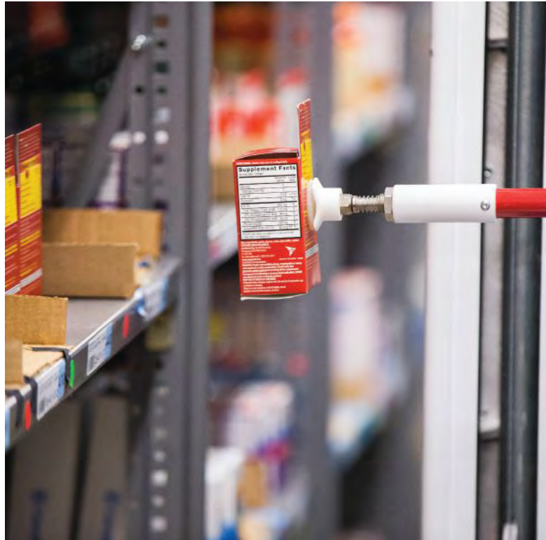
The robot uses a suction cup end effector to pick.
