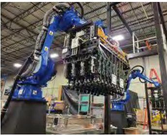
Multi-pick robotic end effector solution processes up to 36 items at a time.
