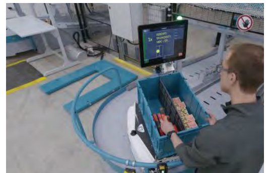
The AMR AS/RS bot moves up the workstation ramp and presents its contents for the operator. The operator’s display reveals the product’s location, SKU description and quantity to pick, as well as where to place it for high accuracy and throughput performance.
