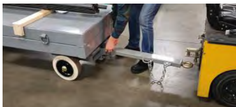
The Tuggable Bar Cart has a removable towbar.
